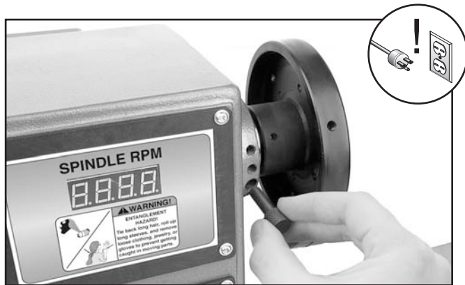
Figure 34. Indexing pin and indexing holes.
